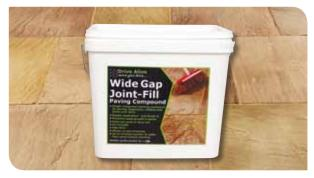
A single component joint filling system for the simple and rapid pointing of paved areas with joints over 5mm. Readyto-use, simple brush application. A unique blend of polymers and aggregates that bind together chemically. On exposure to the atmosphere Joint-Fill forms a stable, solid, mass that is unaffected by the weather once cured. Remains permeable and allows rain water to pass into water course reducing puddling. Eliminates the need for sand/cement pointing!
