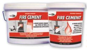
A buff coloured, cement which has a consistency similar to putty. It is resistant to high temperatures and is both air and heat setting. Once cured the mortar will resist temperatures up to 1250°C. Ready to use, blend of high quality clays and selected fillers that sets rock hard when exposed to heat. Does not contain asbestos.
